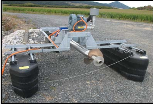
Figure 3-17 Inclined Shaft Aerator
