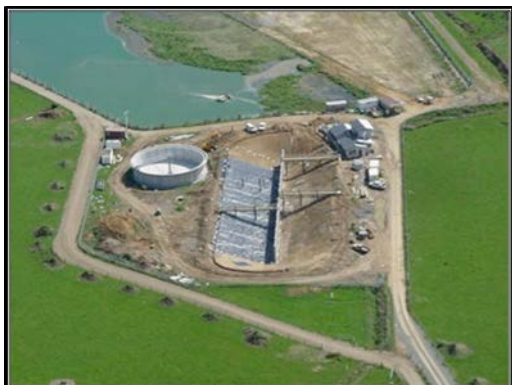
Figure 3-25 Anaerobic Pond Conversion
