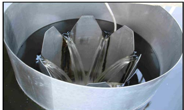
Figure 3-8 Level Control Weir
